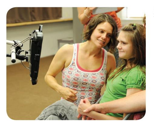
**Indirect selection methods** are supported by some AAC devices. These devices have special software and hardware to interpret input from a source other than a physical keyboard. The most common indirect selection technique is switch scanning. The user selects the message by activating a switch at the moment the desired word, letter, or symbol is highlighted.
