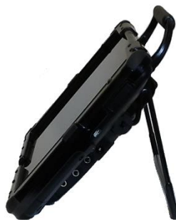
Stand latched in the fully extended position
