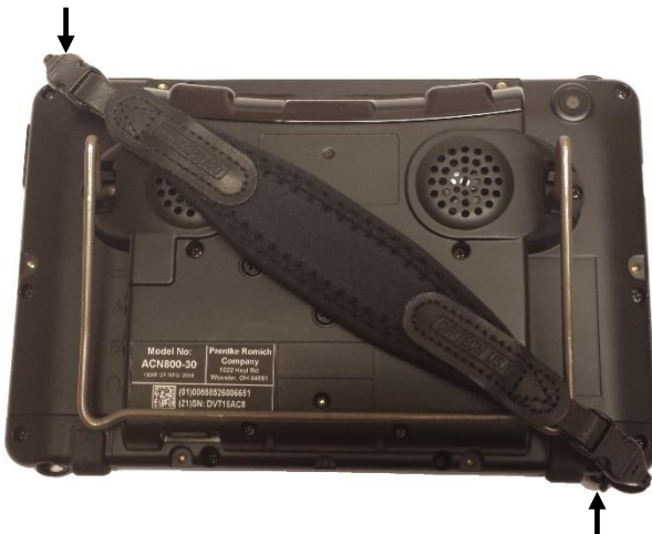
Strap handle attached to strap holder on device
