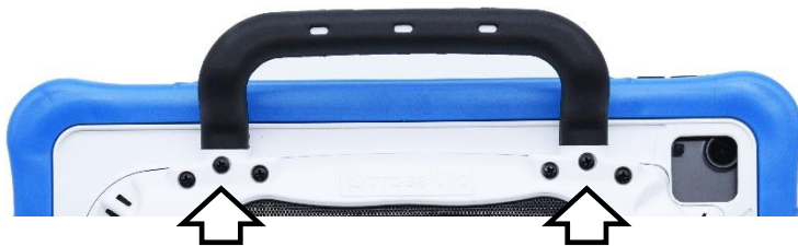
Remove these six screws
